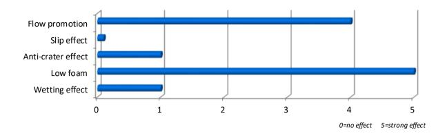
UNIQ \*FLOW P-304 is a cost effective acrylic leveling agent for solvent based and solvent free systems. It's very suitable for gel coats that are base on unsaturated polyesters, epoxides and polyurethanes. The product shows excellent defoaming and leveling performances. It is non-silicone and therefore will not cause intercoat adhesion problems.
